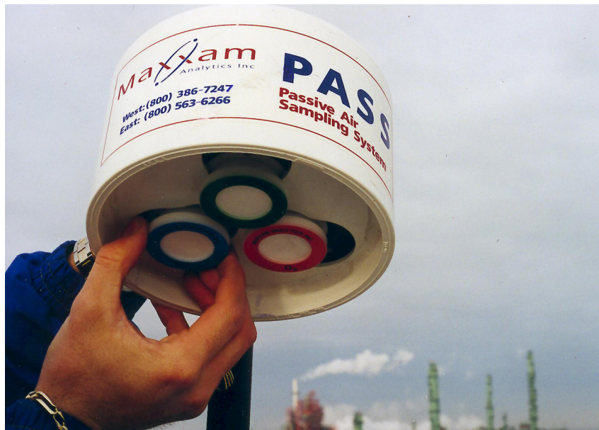
FIGURE 1. Maxxam All-Season Passive Air Sampling System.
