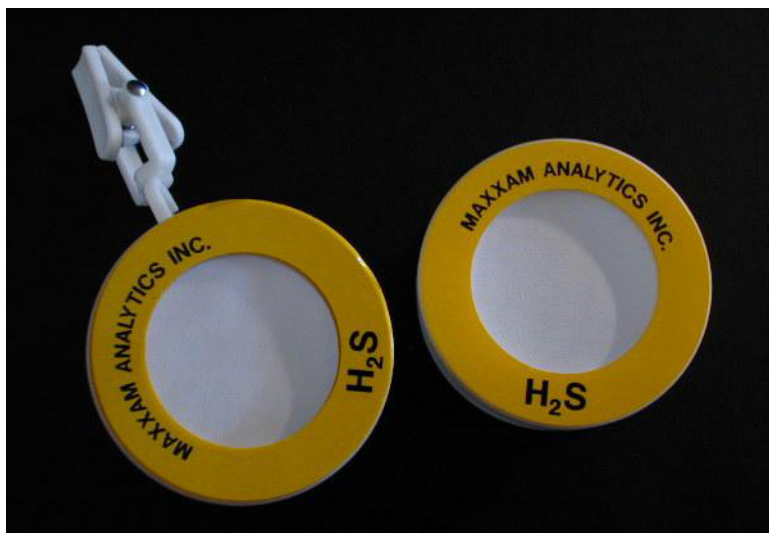
FIGURE 3. Maxxam H 2 S Passive Sampler. The left sampler with a clamp can be used for personal exposure.
